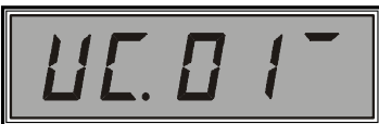
Indication of maximum output level of the active User Chaser in switching mode
