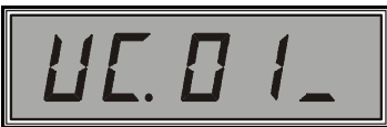
Indication of zero output level of the active User Chaser in switching mode
