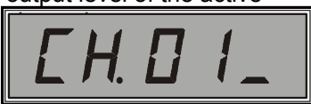
Indication of zero output level of the active channel in switching mode
