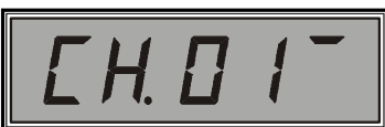
Indication of maximum output level of the active channel in switching mode
